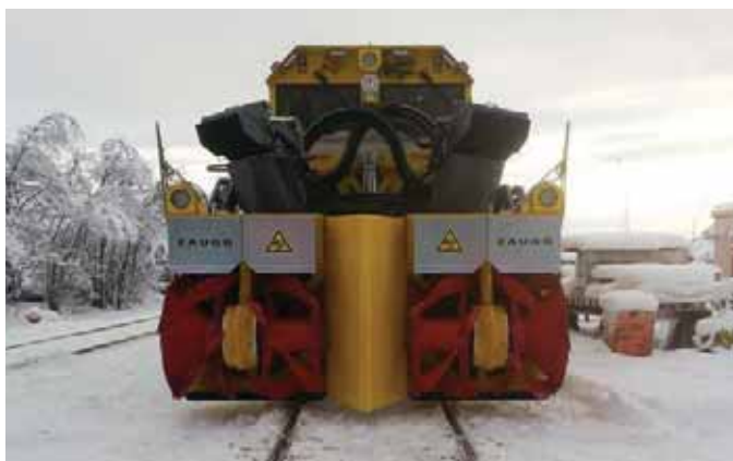
The Zaugg snow clearing vehicle comprises two independent snow blower units at the front, each of which is fitted with an ejection chute for accurate snow ejection. During the first snow blowing pass, the two blowers are retracted together. During the second pass, each one is extended to either side. Between the windscreens there is a high-performance xenon headlight; all other lights are LEDs.
