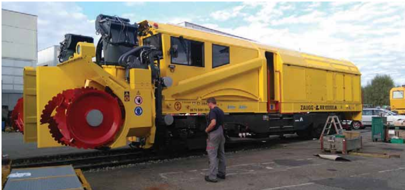
The Zaugg-Matisa self-propelled snow blower locomotive made in Switzerland for Trafikverket, Sweden
