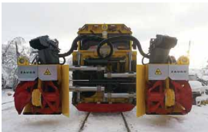
The Zaugg snow clearing vehicle comprises two independent snow blower units at the front, each of which is fitted with an ejection chute for accurate snow ejection. During the first snow blowing pass, the two blowers are retracted together. During the second pass, each one is extended to either side. Between the windscreens there is a high-performance xenon headlight; all other lights are LEDs.
