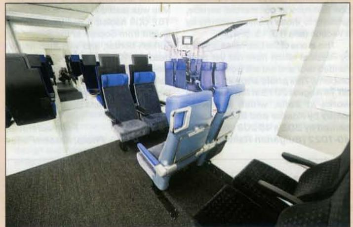
On the left, the mock-up of a first class saloon. Here the distance between seat backs is a generous 2,040 mm. The right-hand photo shows the mock-up of a second class saloon. In seating bays the distance between seat backs is 1,850 mm, while in rows it is 860 mm. Both in first and second class the seats are adjustable/reclining. Significantly a clear window view, unobstructed by window pillars, is provided from each seat.
