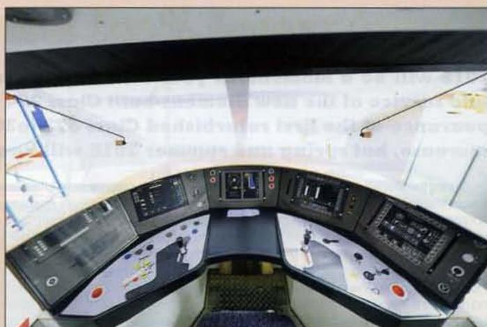
The design of the Giruno's driving console is based on that of the FLIRT and KISS EMUs.
