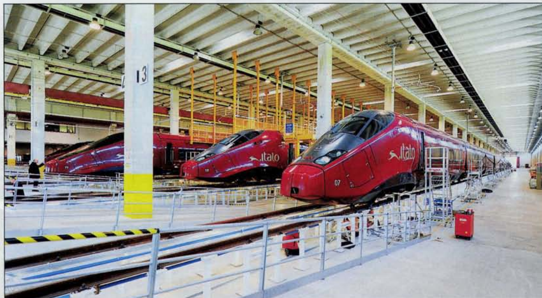
AGVs 07, 18 and 19 on 8 November 2012 in Nola depot, near Napoli, where Alstom realises maintenance on NTV's Class ETR 575 trains under a 30-year contract.
