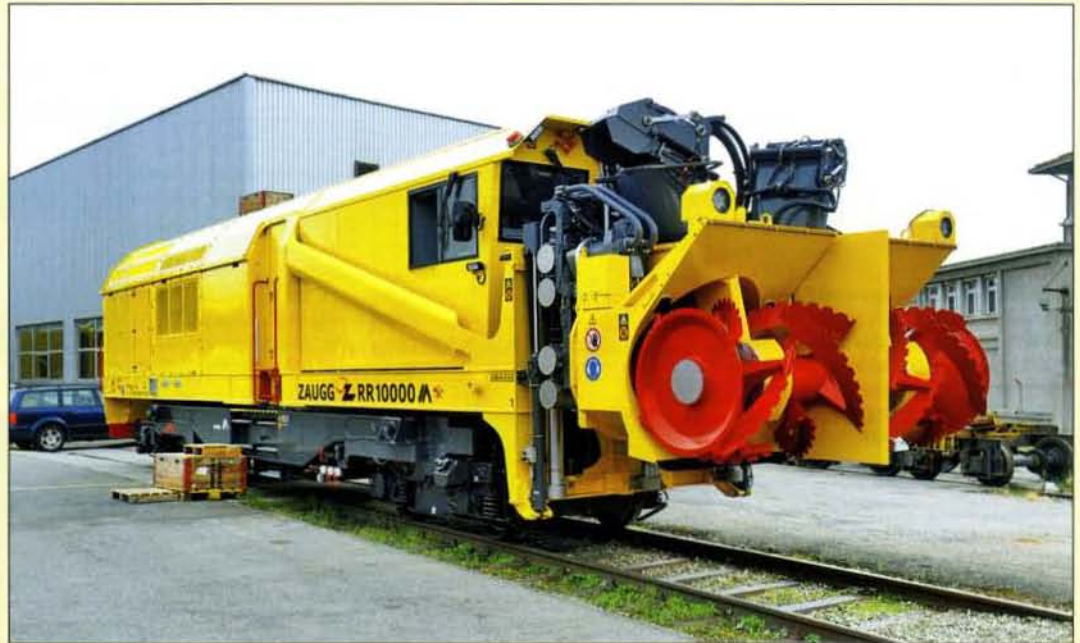
The upper view shows snow-blowers in the retracted position, and raised for running on lines where snow clearance is not required. This position also ensures that the discharge chutes do not exceed the loading gauge. This photo was taken on 13 October 2015 at the Matisa factory at Crissier. The machine EVN is 99 74 9491 001-8.
