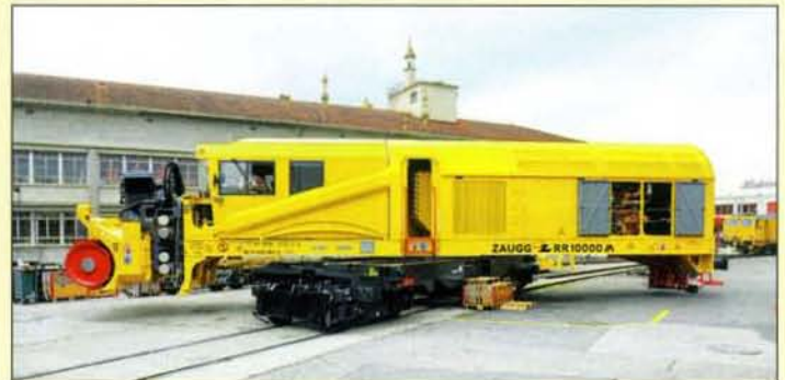
A side view, showing how the bodywork can be rotated on the turntable ring mounted on the underframe. The door to the engine compartment is open. The snowplough will be installed at the same end as the engine compartment following delivery to Sweden.
