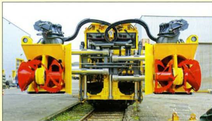
Ready for action! Here the snow-blowers have been extended on either side to the vehicle to their maximum outreach position. A high-powered xenon searchlight is provided in the centre, between the blowers, but all other lights have LEDs. Some of the lights are only intended for use during maintenance.
