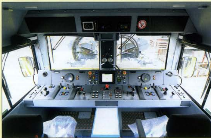
A view of the driving console. Both windcreens are fitted with heating wires. At each driving/operating position the air brake lever is on the left and the traction control lever on the right. The snowplough is operated using buttons situated between the brake and traction controls. In front of these buttons there are two joysticks used for the snow blowers.
