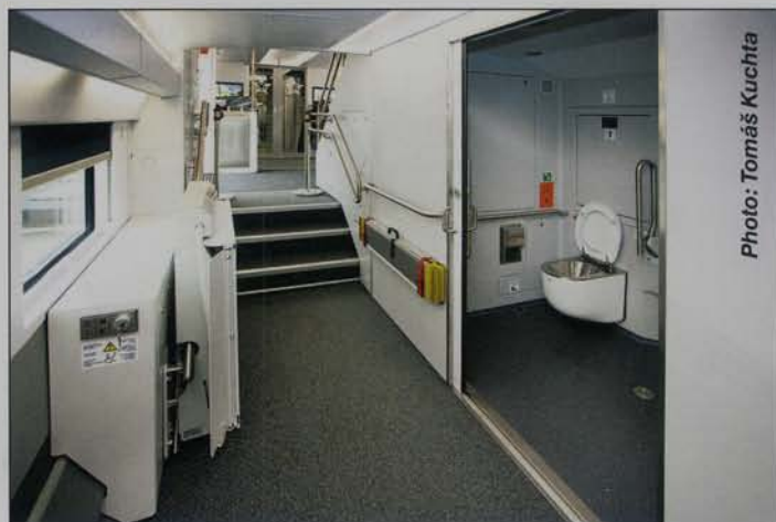
The end car with economy class seating also has a dedicated area for handicapped passengers. Here the wheelchair-accessible WC cubicle is situated on the lower deck, adjacent to the entrance vestibule. On the left is a wheelchair lift, for the short flight of stairs.
