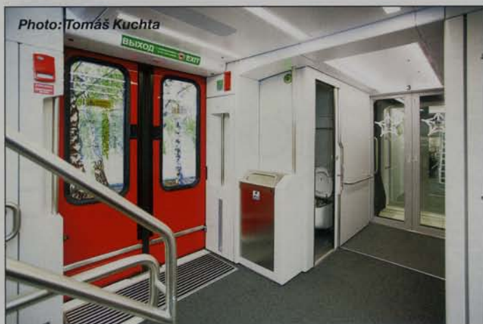
The WC cubicles are also located on the mezzanine decks. This is a standard-sized cubicle. Note the inter-car gangway beyond.
