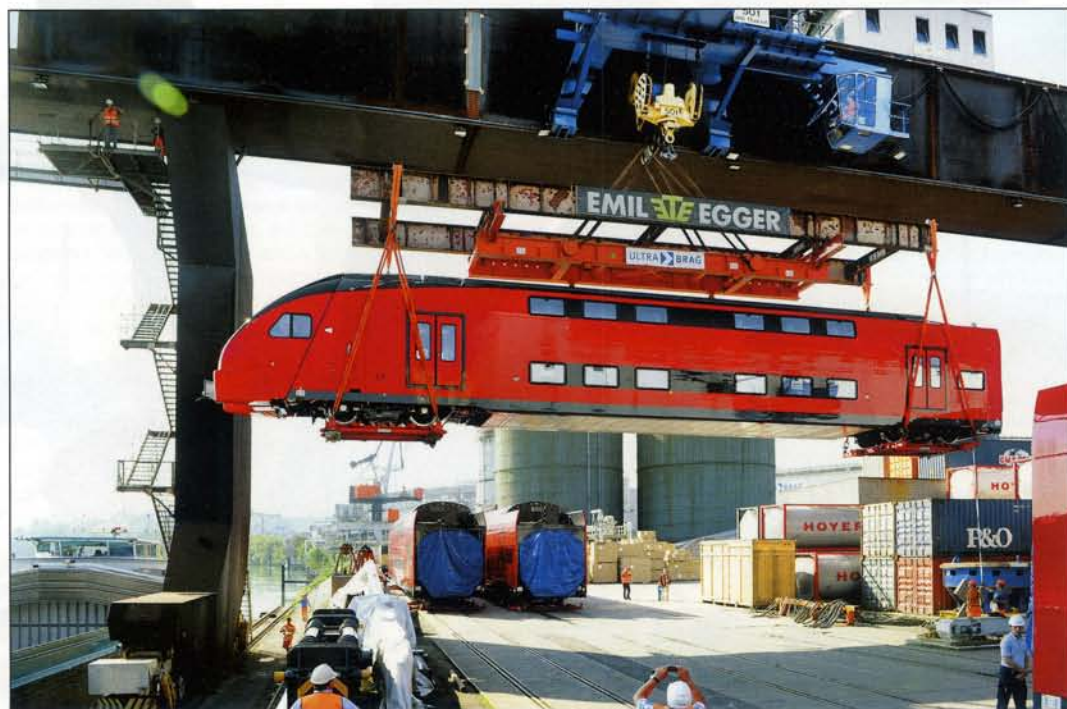
The 2,430 km delivery journey from Switzerland to Belarus, preparations for which took during the 13 months before the first batch of cars were moved to Fanipol, was an exceptionally complicated one, on account of the huge size of these double deck trains. This eliminated all possibilities of moving the vehicles by rail across Europe on 1,435 mm gauge tracks. Starting at Stadler's Altenrhein works, the cars of ESh2-001 KISS were moved, one by one, on low-loaders to the Rhein port of Auhafen in Muttenz, in the southeastern suburbs of Basel (see R 5/14, pp. 54 - 55). At Muttenz the cars were mounted on their 1,520 mm gauge bogies, and stored on specially designed pallets, which enabled them to rest on the quayside or on the deck of a vessel (see photo, taken on 6 September 2014).
