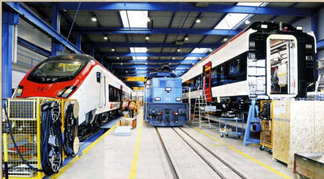
Two halves of the first Giruno at the IBS on 16 February 2017. The blue Class Eea shunter, 97 85 1936 133-8, is used for haulage of new stock between Bussnang and Erlen. Note the dual gauge track (1,435/1,000 mm), necessary for testing new trains, especially for the Swiss market.
