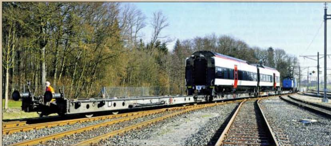
On 16 February 2017 the Class Eea shunter, running on battery power, shunts the 6th and 7th bodyshells for the first Giruno into the smaller hall at Erlen for mounting on bogies and coupling up to the rest of the train.
