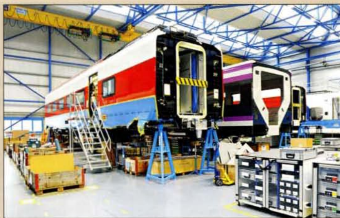
Final assembly of the Giruno cars at Stadler Bussnang factory on 15 February 2017. On the right is a bodyshell for one of the Junakalusto FLIRTs.
