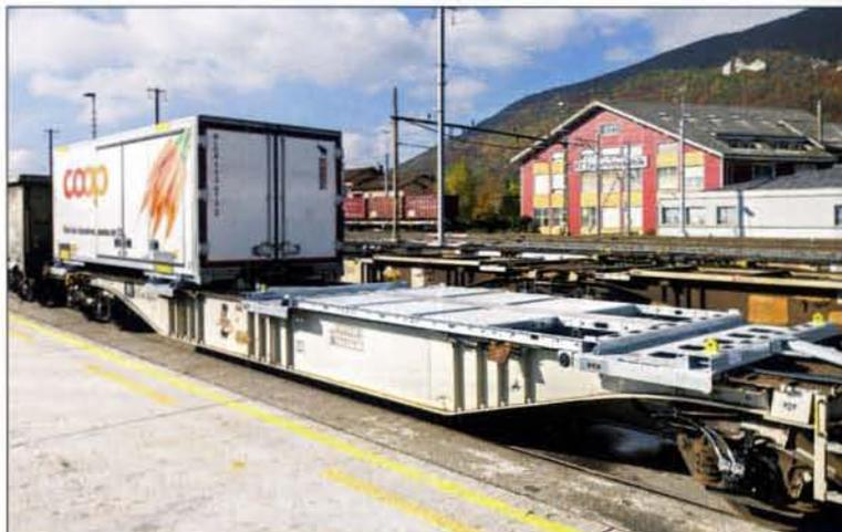
*The upper photo shows a typical example of RailCare's transport system. This is an articulated platform wagon fitted with a ContainerMover 3000 frame adaptor. On the left a swapbody is being loaded. The frame adaptor has been fitted with six square panels housing six batteries and there are two empty spaces, which could be filled with two more batteries.*
