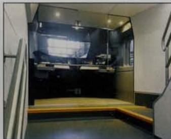
views of the passing scenery. The wheelchair harness points will be located close to the entrance doors, and the latter will be fitted with retractable steps and ledges to bridge the horizontal and vertical gaps between train floor and platform. Capacious luggage storage spaces will be provided, together with facilities for bikes.
