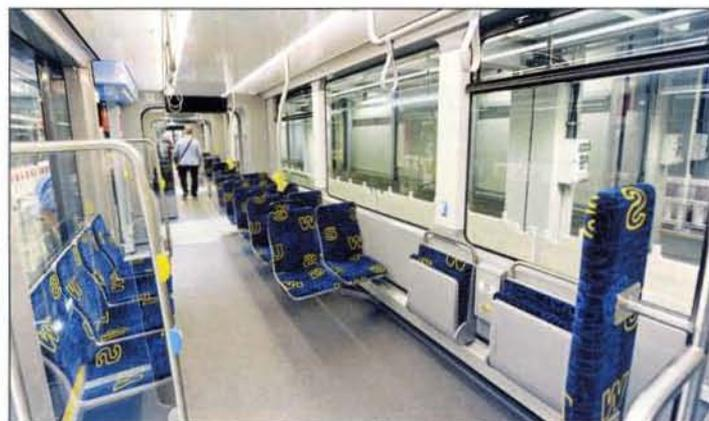
of the end sections. The interiors are fitted with HVAC, and have two large multi-purpose areas, suitable for prams and wheelchairs. **Seats are provided for 69 passengers, and space is available for up to 116 standees at a density of four per m². The lower photos show driver's cab arrangement, and an auxiliary driving console in the rear section of the tram.**
