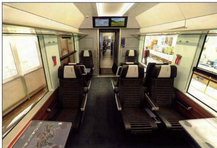
**35 seats, with 2,050 mm between seat backs, mostly in 2 + 1 bays, with 1,800 mm between seat backs, in 2 + 2 configuration, and also in bays. 18 tip-up seats are also provided, and there is room for up to 179 standees.**
