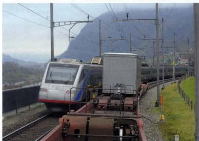
Below: Locomotive ES 64 F4-088 hauling two Modalohr tandem wagons after leaving the Wattingen tunnel en route from Airolo to Arth-Goldau (photo: A. Schmutz).
