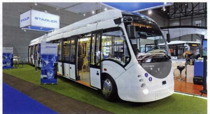
Above: The trolleybus "Vitovt Max Duo 43303A", built in Minsk with diesel auxiliary drive, at the Stadler stand. However, there is no evidence of the Swiss manufacturer on the bus itself (photo: J. Lüthard).
