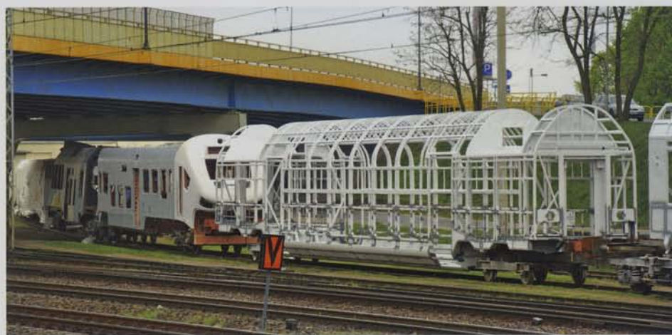
Below: Body shell of a double-deck coach on the vehicle manufacturer Pesa premises at Bydgoszcz (photo: S. Karkowski, 1 May 2015).
