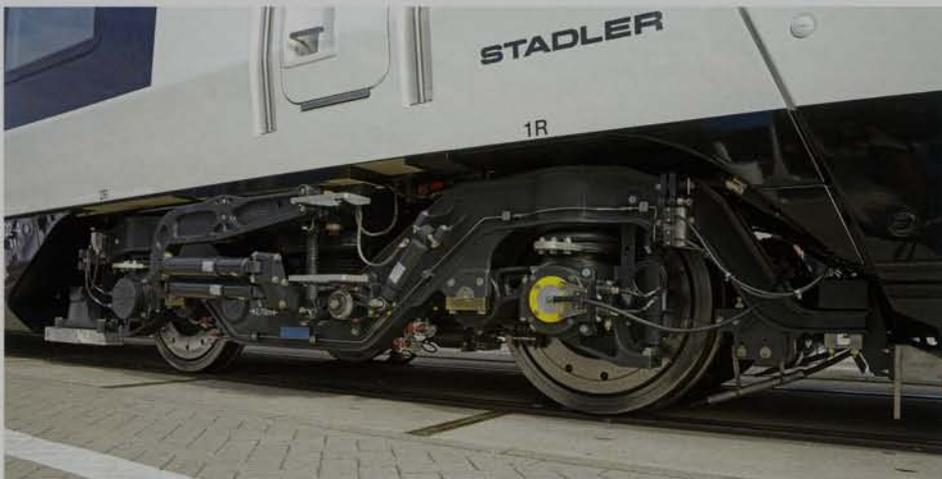
Left centre and below: The powered bogie in the end car as well as an unpowered Jacobs bogie between two coaches of the Giruno (photos: A. Gerber).
