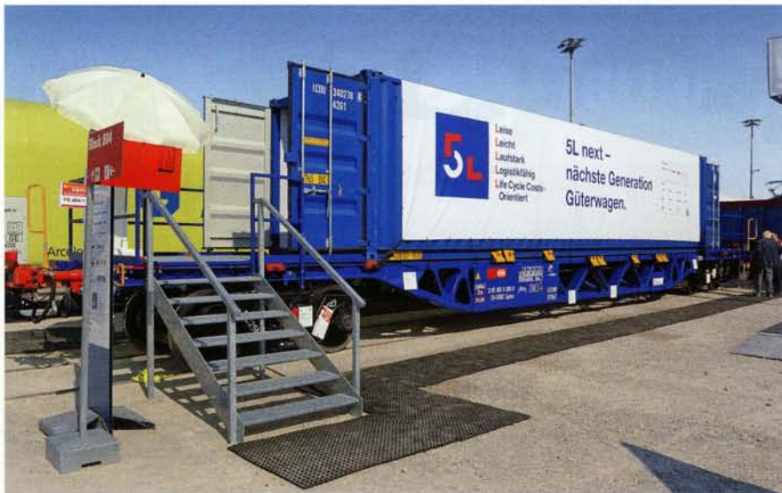
At the Transport Logistic 2019 trade fair in Munich in early June, SBB Cargo showcased a Sgnss freight wagon with a riveted and bolted rather than welded middle segment and radially adjustable wheelsets. The tare weight of the wagon is 15.6 t, according to its markings. The company is working together with VTG and Hupac on this project (photos: J. Lüthard).
