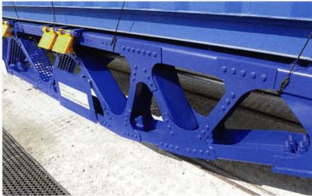
At the Transport Logistic 2019 trade fair in Munich in early June, SBB Cargo showcased a Sgnss freight wagon with a riveted and bolted rather than welded middle segment and radially adjustable wheelsets. The tare weight of the wagon is 15.6 t, according to its markings. The company is working together with VTG and Hupac on this project (photos: J. Lüthard).
