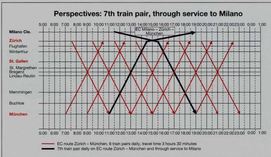
The Astoro trainset will operate only individually, as the stations in the Allgäu do not have any platforms long enough for 374-metre double composition trains (see box on the next page). For the 17.33 connection from Zürich, a double unit is required for commuter traffic services from Zürich to St. Gallen, as outlined above.
